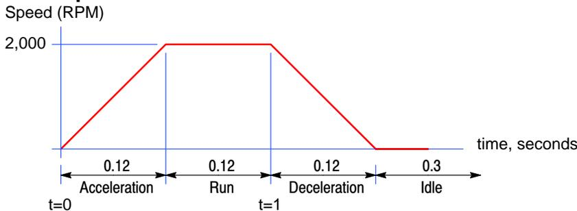
As friction and torque are overcome, the motor and load begin to accelerate. As the motor approaches the commanded speed, the error signal is reduced and, in turn, voltage applied to the motor is reduced. As the system stabilizes at running speed, only nominal power (voltage and current) are required to overcome friction. At t=1, the load approaches the desired position and begins to decelerate.
