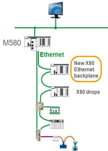
**Ethernet Backplane Provides Connectivity and System Flexibility, so Adding or Modifying Drops Can Be Done On The Fly**
