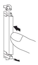
As soon as the CF-card is inserted the MCPWR and BUSY indicators will go ON.
