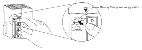
Press the Memory Card eject button after the BUSY indicator is no longer lit.
