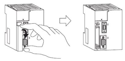
Insert the Memory Card with the label facing to the left. (Insert with the Δ
