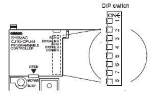
MCPWR indicator will go ON and BUSY indicator will flash. BKUP indicator on the CPU unit will flash a few times as well. Wait until all 3 mentioned indicators are OFF.
