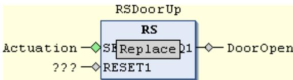
As there may be three possible reasons to stop the opening process of the garage door, we will place an OR operator (three inputs) in front of the RESET1 input of the RS block. All three reasons are queried and connected to the inputs of the OR operator:
