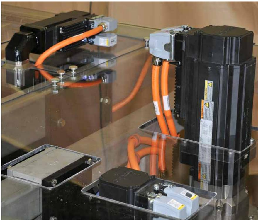
With Rexroth's IndraDrive Mi integrated motor/drive system, multiple drives are daisy-chained together and share power from the same bus, significantly reducing energy consumption.
