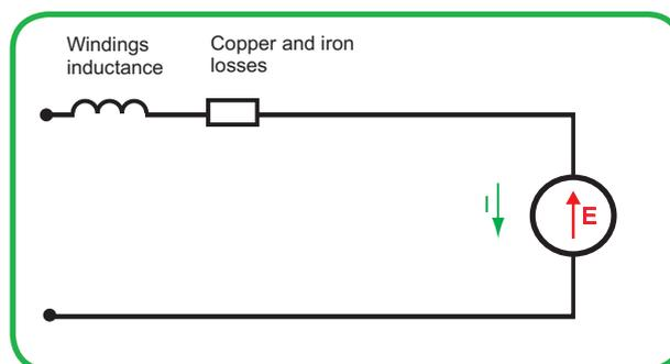
$E$  is an image of the electromotive force of the machine which depends on flux, created by the magnets and the number of revolutions  $\omega$ .
