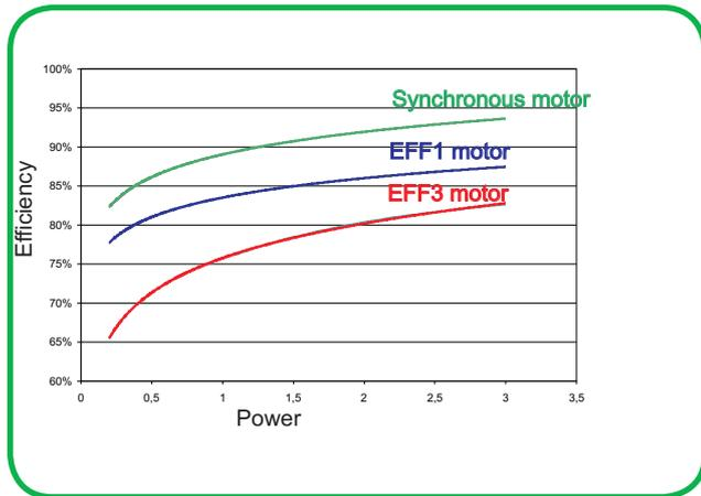
Part of AC motor weakness disappears, in particular the power-factor.
