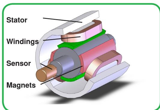
The stator has an embedded three-phase winding.
