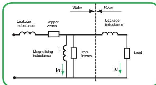
If we neglect the windings resistance, we see that the voltage applied to the magnetizing coil noted L creates a current named  $I_0$ .
