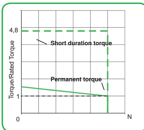
Its nominal torque is 5,2 Nm at 3000 rpm which produces 1.6kW.
