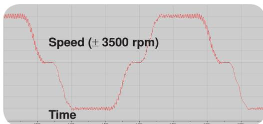
Test with a 50kg. load
