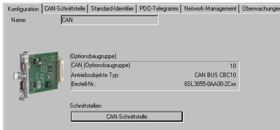
In the "CAN interface" tab, you can set the transmission speed ("baudrate") and the node ID ("CAN bus address").
