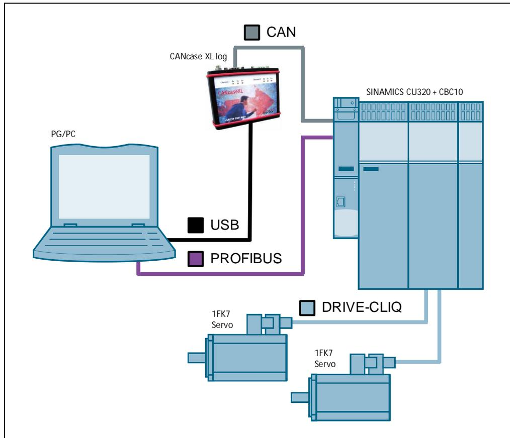
In this application description it is shown, how a SINAMICS drive can be moved speed-controlled by means of the CAN interface "CANcase XL log".
