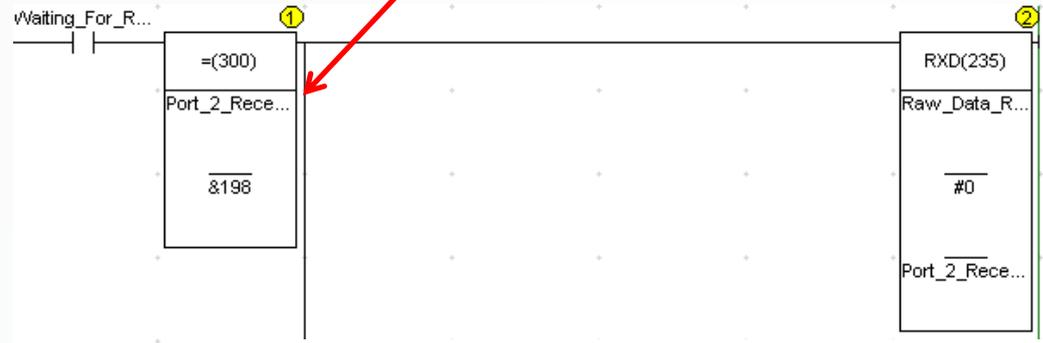
This is the PLC receive function block, this block moves 198 bytes of data to the PLC DM registers starting with DM200.
