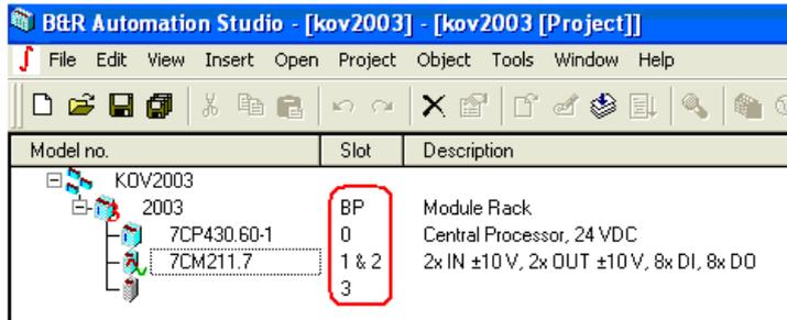
Fig. 7.6: Hardware configuration in the B&R Automation Studio.
