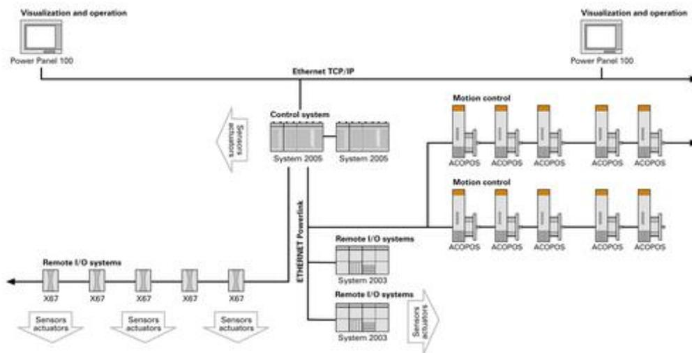
Fig. 7.4: Communication network with B&R System 2005.
