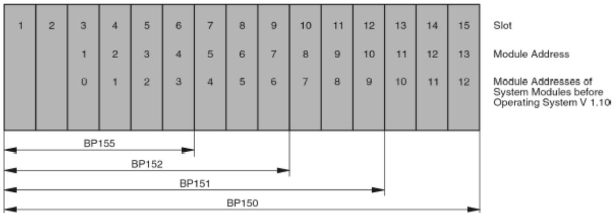
Fig. 7.7: Maximum expansion B&R System 2005 and its address in slots.
