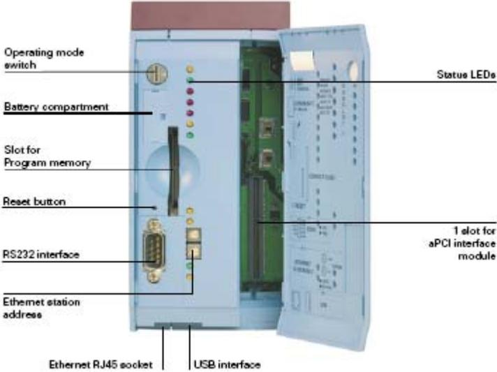
Fig. 7.3: Central processor unit CP360.
